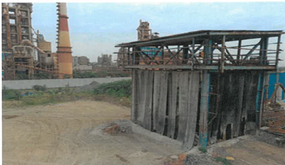
Belt curtains provided at crusher hopper
